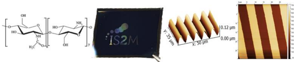
Figure 1 : Molecular structure of chitosan, examples of patterns obtained by DUV photolithography and after transfer by reactive ion etching (AFM).
